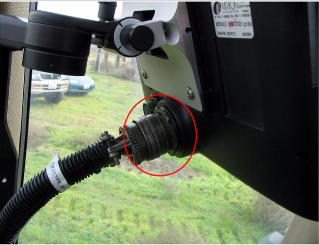
A close-up photograph of the back of a black user terminal. A black cable with a multi-pin connector is plugged into a port. The connector is circled in red. A white label on the cable reads 'INFO-TYPE'. Above the terminal, a small white sticker is visible with the text 'MINKON', 'MODUL 480001 prota', and 'S/N Nr. 00012 40224'. | Das Kabel auf der Rückseite des Anwenderterminals anschließen.                     |
