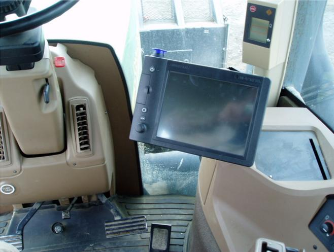
A photograph of the operator's seat in a vehicle. The user terminal is mounted on the dashboard in front of the seat. The terminal has a screen and several buttons. The interior is beige and tan. The window shows a green field outside.                                                                                              | Den Anzeigewinkel einstellen. Die Abbildung zeigt das Terminal nach dem Anschluss. |
